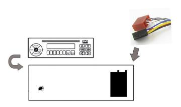
5 Finally, connect the white female Mitsubishi connectors to the corresponding male connectors in the vehicle.
